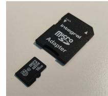
Option 2: Zafena provides a link to download the latest software to a PC. The workstation's micro-SD card is mounted in the PC. The downloaded software is transferred to the card (contact Zafena for instructions) The Micro-SD card is remounted in the workstation.
