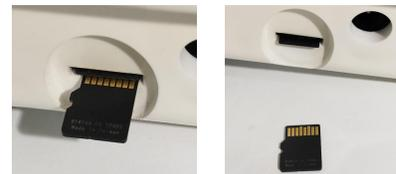
4. Install the new memory card in the same slot as the old one, with its golden contacts facing up. Insert it in a slightly upward position. The card must be hooked into a holder and lowered completely into the card slot.
